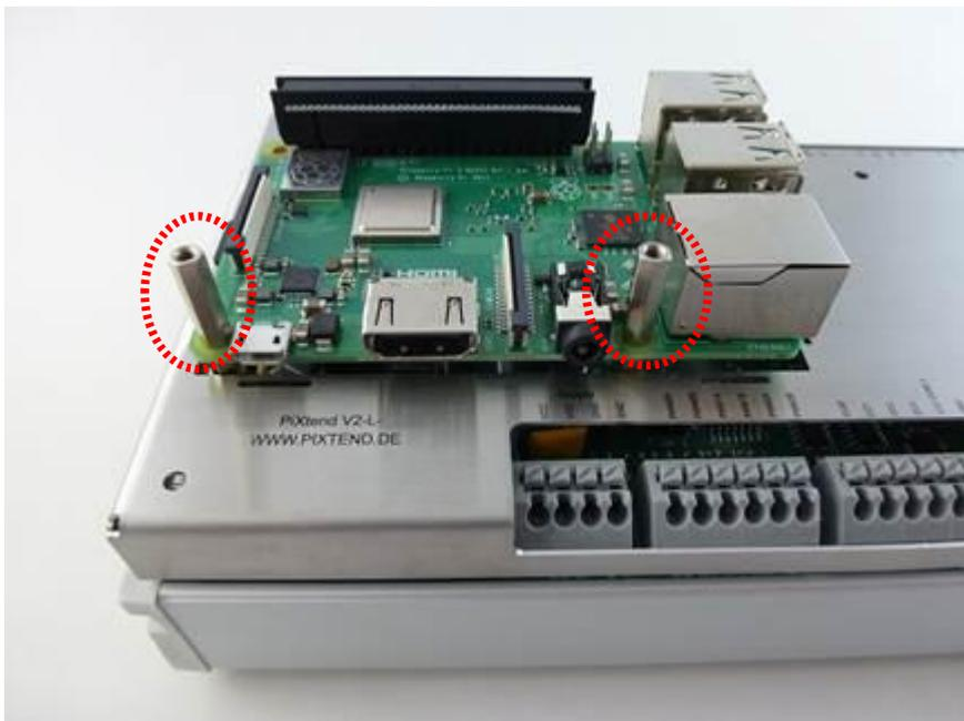
Figure 21: Two spacers screwed into the Raspberry Pi
