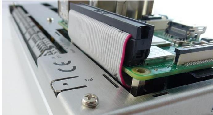
Figure 23: Optimal routing of the ribbon cable
