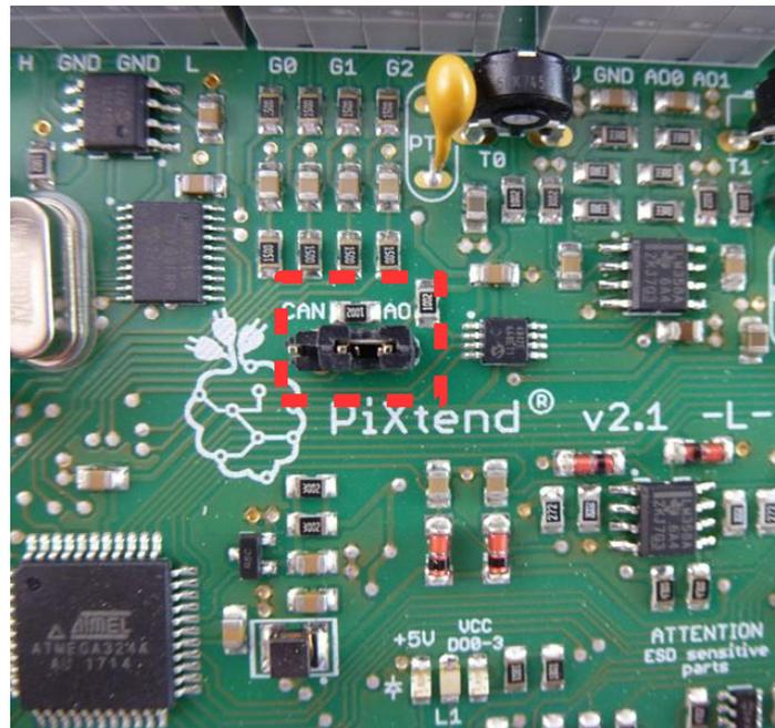
Figure 35: Jumper – AO/CAN – set to AO
