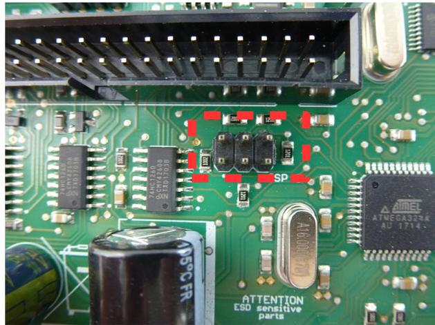
Figure 52: ISP 0 connector - In-System-Programming (ISP) - ATmega324A
