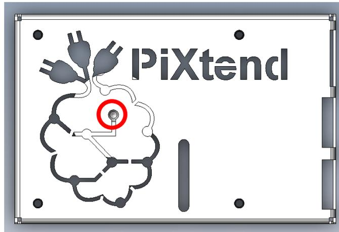
Use one of the M2,5 x 6 mm screws to fix the heatsink to the upper cover part, creating one single part.
