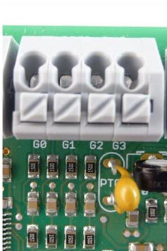
Figure 66: Terminal block connection - GPIOs
