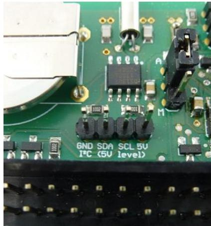
Figure 47: Pin header - I<sup>2</sup>C on 5V level
