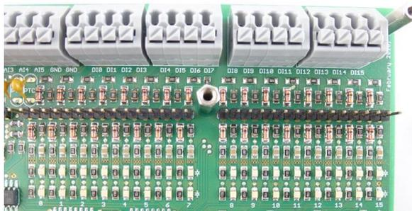
Figure 58: Terminal block - digital inputs
