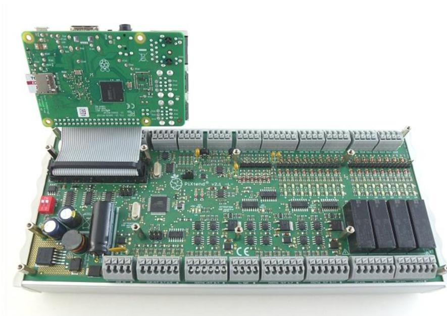
Figure 19: Raspberry Pi unscrewed from the PiXtend
