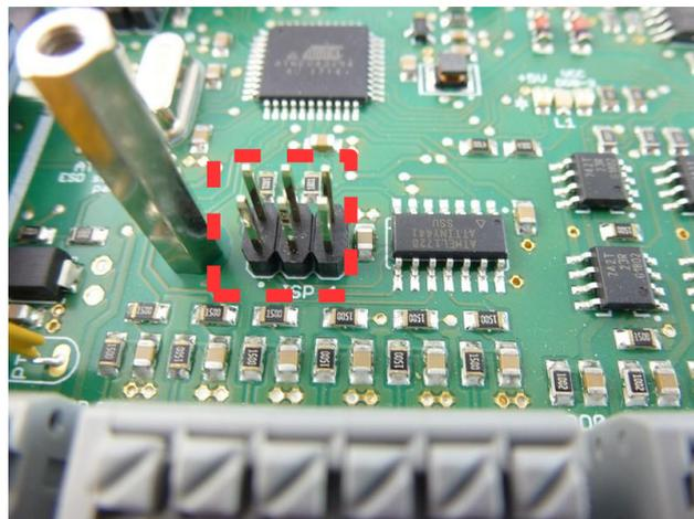
Figure 53: ISP 1 connector - In-System-Programming (ISP) - ATtiny441
