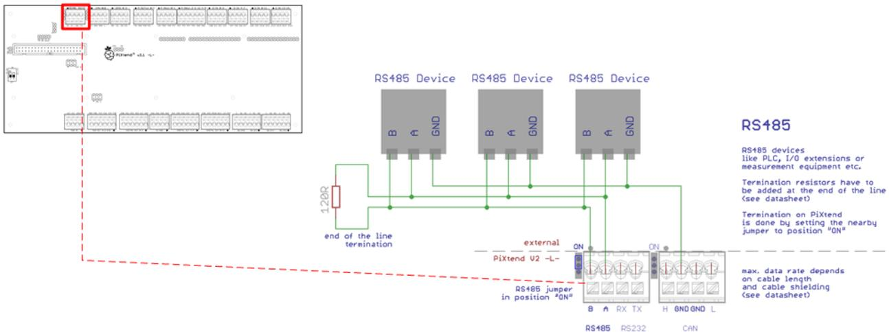
Figure 83: Simplified wiring diagram: connection of the RS485 interface
