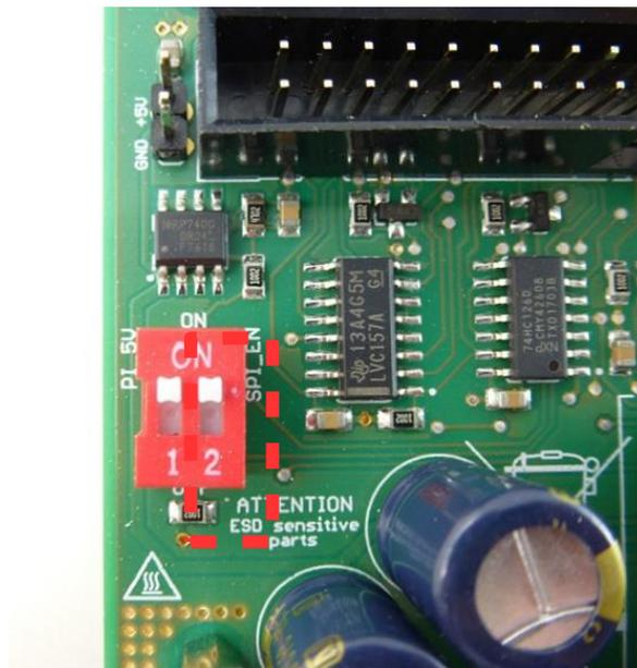
Figure 28: Switch – “SPI\_EN”
