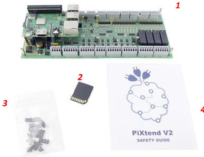
Figure 4: Package contents - PiXtend V2 -L- ePLC Basic/ePLC Basic
