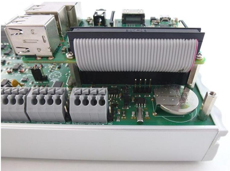
Figure 45: Connection between the PiXtend V2 -L- and Raspberry Pi
