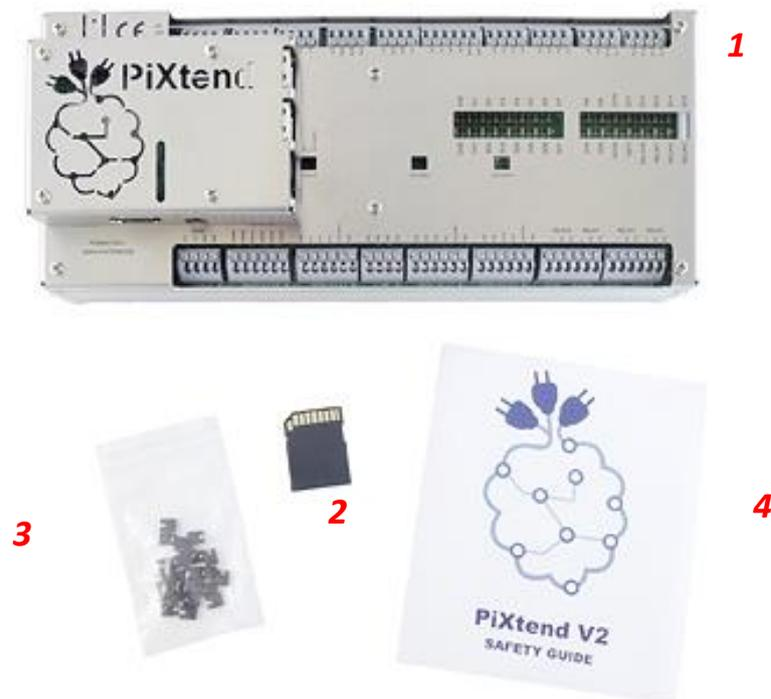
Figure 5: Package contents - PiXtend V2 -L- ePLC Pro/ePLC Pro Pi4
