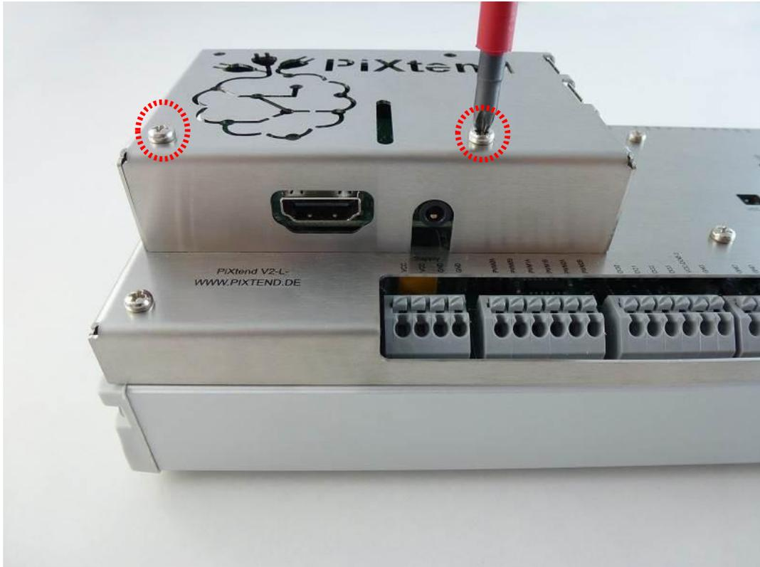
Figure 25: First step of mounting the upper cover
