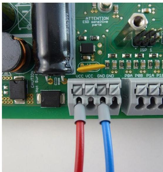
Figure 39: Power connection to the PiXtend V2 -L-
