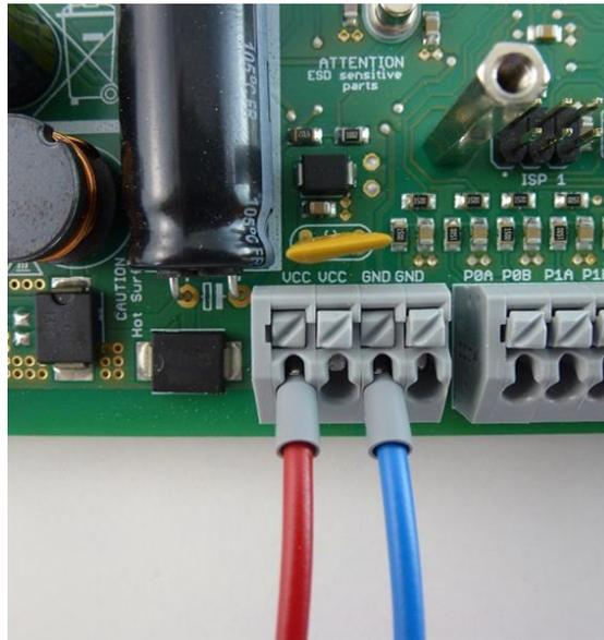
Figure 43: Terminal block for the power supply
