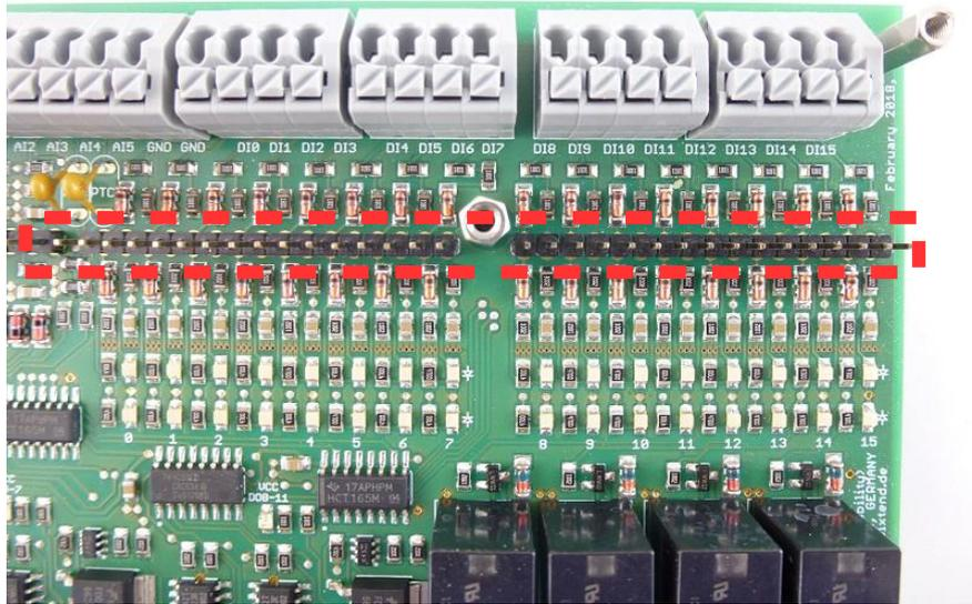
Figure 31: Jumper - digital inputs in 24V range (factory default)
