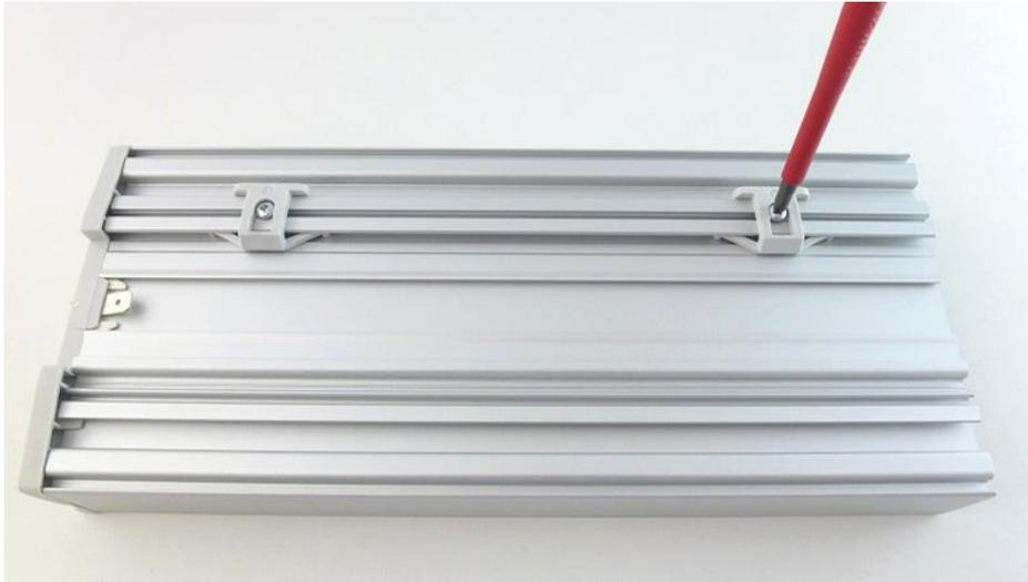
Figure 12: Screwing the locking brackets into place
