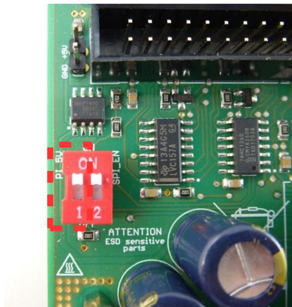
Figure 29: “PI\_5V” in the “ON” position
