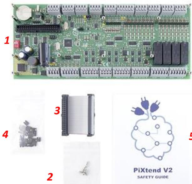
Figure 1: Package contents - PiXtend V2 -L- Extension Board (Article number 50199 001)
