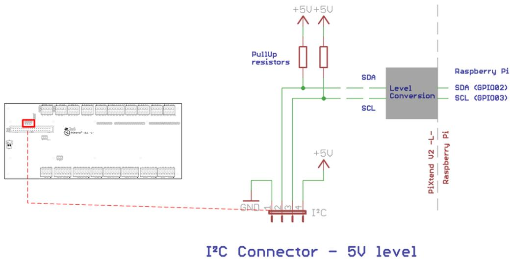
Figure 48: Simplified wiring diagram: I<sup>2</sup>C at 5V level
