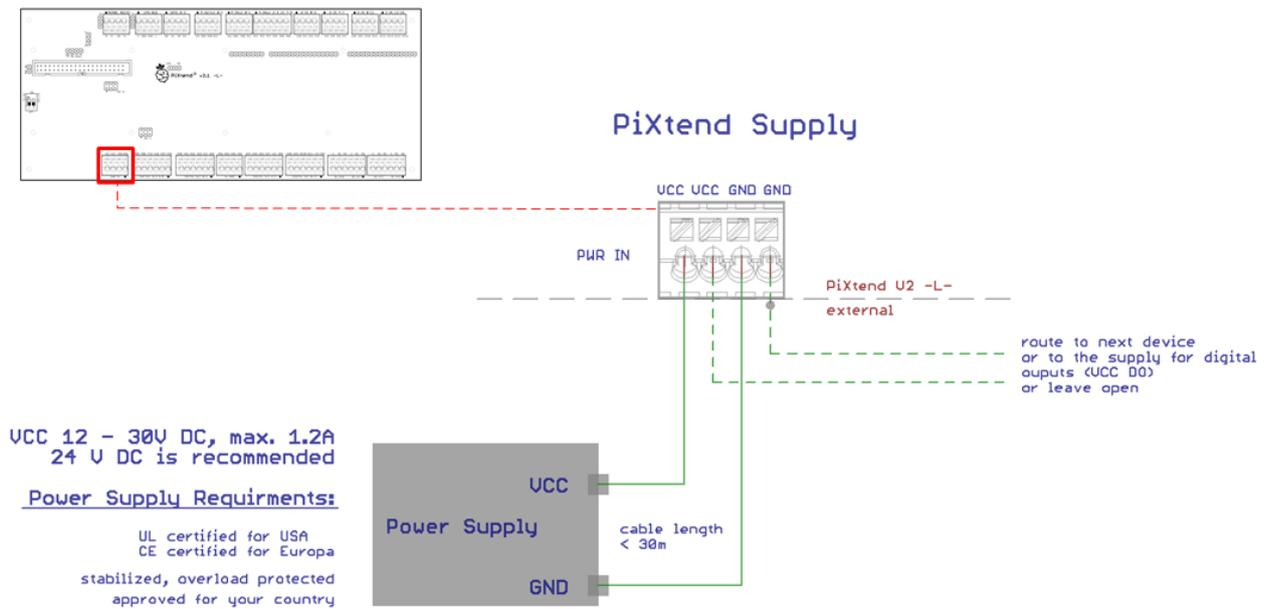
Figure 44: Simplified wiring diagram: power supply connection
