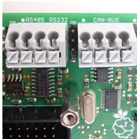
Figure 81: Terminal block connectors - serial interfaces
