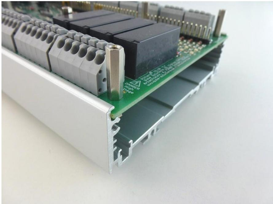
Figure 13: Connecting the PiXtend and housing profile together
