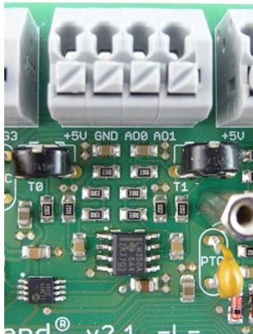
Figure 75: Terminal block - analog outputs
