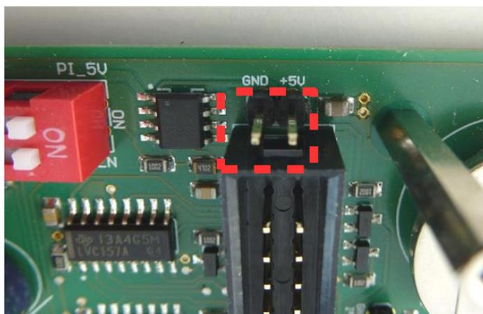
Figure 49: Power supply connection - Raspberry Pi 7" touch display
