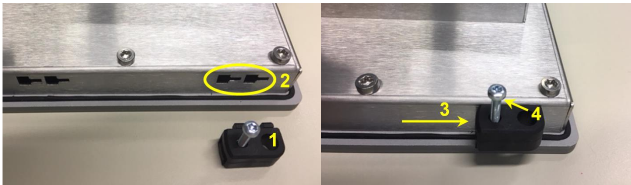
Figure 5: Mounting in control cabinet front for panels up to 7" display size
